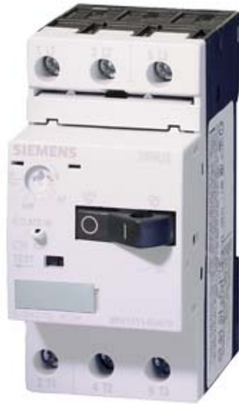
CIRCUIT-BREAKER SIZE S00, FOR MOTOR PROTECTION, CLASS 10, A-REL.0.45...0.63A,N-REL.8.2A SCREW TERMINAL, STANDARD SWITCHING CAPACITY
